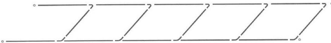
**Step#4** – Attach the pipe lengths to the 90° fittings using the set screw and your Allen wrench. Also attach the 10 ea. feet to the now completed "U" frames.
