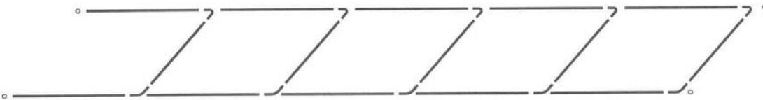
**Step#4** – Attach the pipe lengths to the 90° fittings using the set screw and your Allen wrench. Also attach the 10 ea. feet to the now completed "U" frames.
